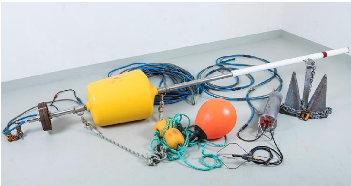
Figure 2: Hydroacoustic online monitoring system.
